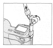
A neckstrap is supplied with your Maxxum 8000i for easy carrying. Attach it to the camera as shown above. An eyepiece cap is also sup-
