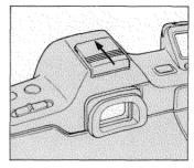
The eyepiece cap slides over the eyepiece to prevent stray light from entering the camera and affecting exposure. It should be used whenever the eyepiece is not shielded by your head, as when using the self-timer or when operating the camera by remote control. To attach the eyepiece cap, first remove the eyepiece cup, then slip the cap over the frame.
